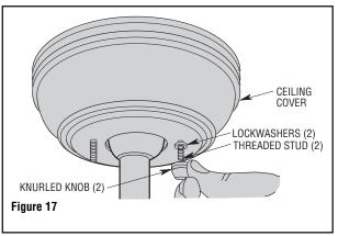
5. Secure the ceiling cover in place by sliding lockwashers over the threaded studs and installing the two knurled knobs (supplied). (Figure 17.) Tighten the knurled knobs securely until the ceiling cover fits snugly against the ceiling and the hole in the ceiling cover is clear of the downrod. Your fan is now wired to be turned on and off from the fan switch.
